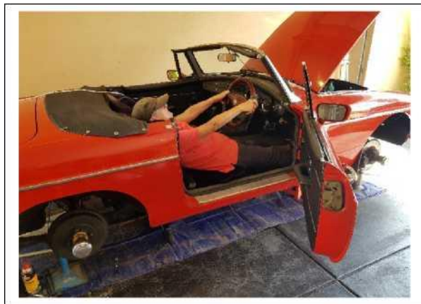
The 'Director of Works' assisting with the bleeding of the brakes. Note how easily she reaches the pedals, height is an advantage.
